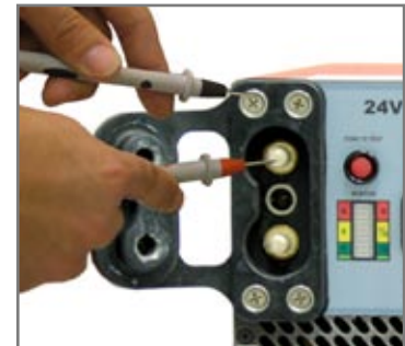
3.8.6 - DC Output Connector Negative Pin
