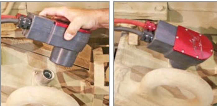
Figure 3.11.2 Attaching NATO DC Power Cable to vehicle
