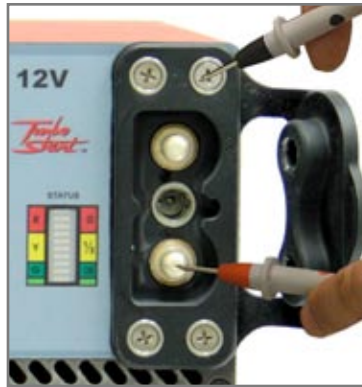
3.8.3 - DC Output Connector Positive Pin
