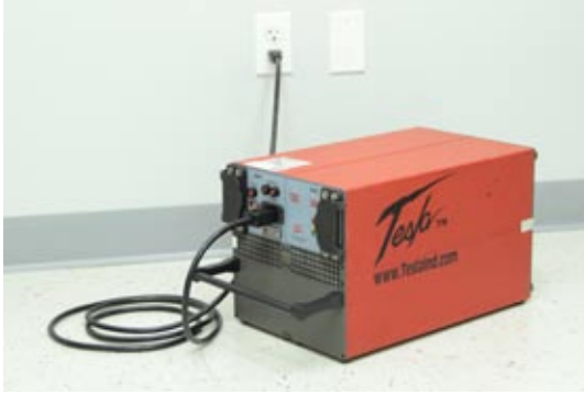
Figure 3.12.1 - Connecting TI1560 12-24 GPU to AC Power Supply
