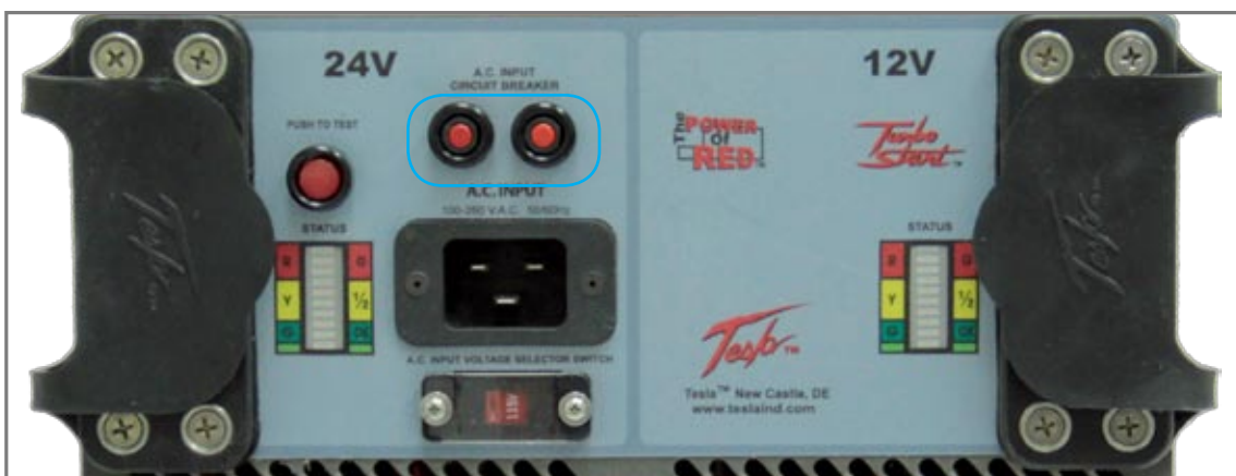
Figure 2.8.1 - AC Input Circuit Breaker (outlined in blue)
