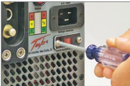
Figure 2.12.2 - Unscrew Protective Cover
