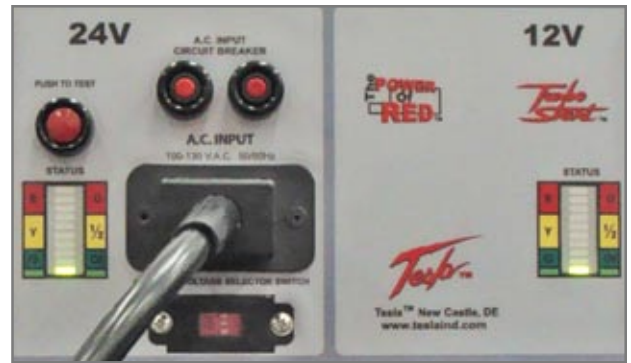
Figure 3.12.2 - AC Power Connected with LEDs Illuminated
