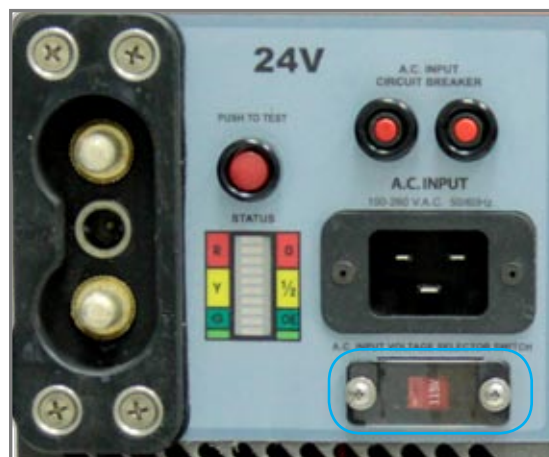
Figure 2.12.1 Input Voltage Selector Switch (outlined in blue)
