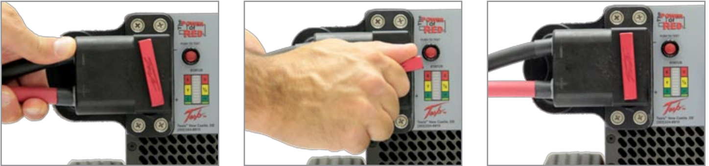
Figure 3.11.1 Attaching DC Power Cable to GPU
