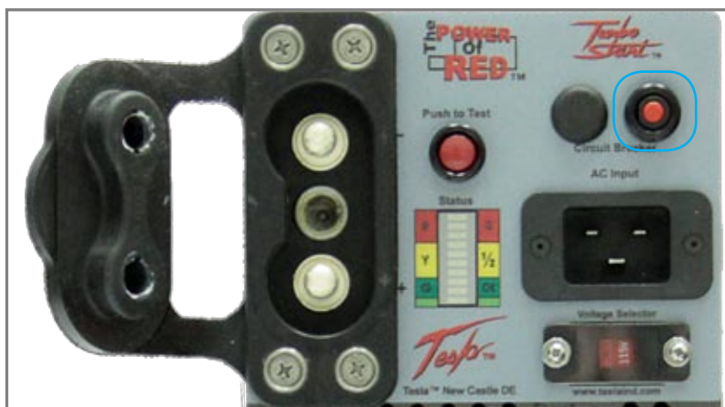
Figure 2.8.1 - AC Input Circuit Breaker (outlined in blue)
