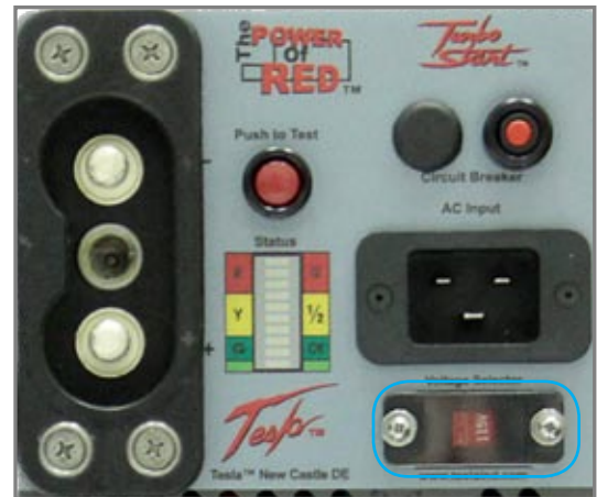
Figure 2.10.1 Input Voltage Selector Switch (outlined in blue)
