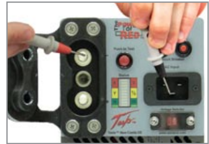
3. Move the positive probe to the dc negative post. Multimeter should read greater than 10 M \Omega .
