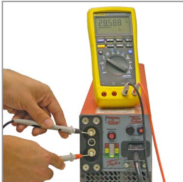
Figure 3.8.2 – Testing DC Receptacle
