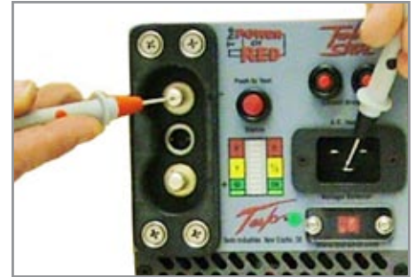
3. Move the positive probe to the DC negative post. Multimeter should read greater than 10 MΩ.
