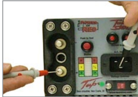
2. Place the negative probe on the ac ground post and the positive probe to the dc positive post. Multimeter should read greater than 10 MΩ.
