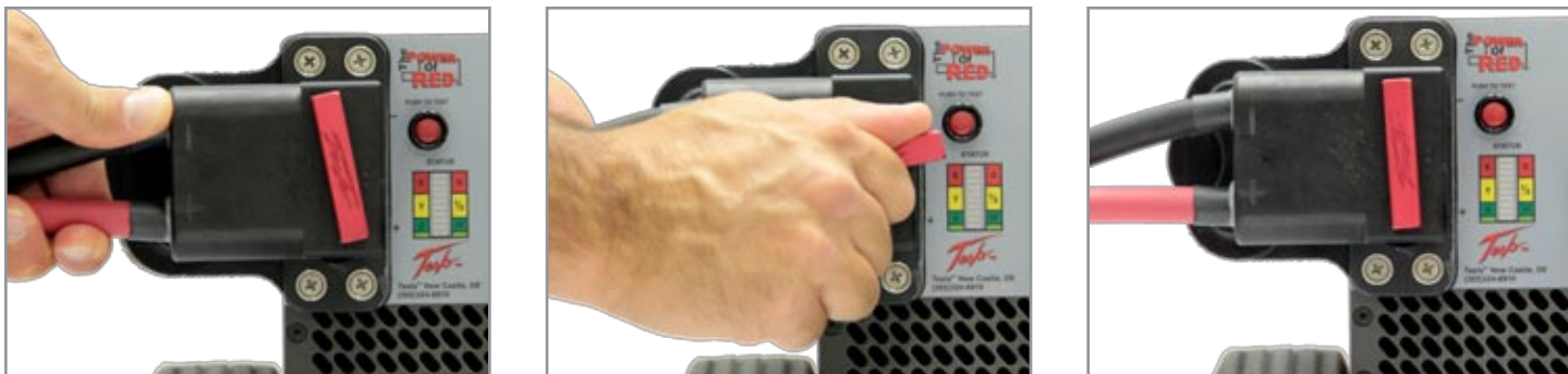
Figure 3.11.1 - Attaching DC Power Cable to TI2500 GPU-24
