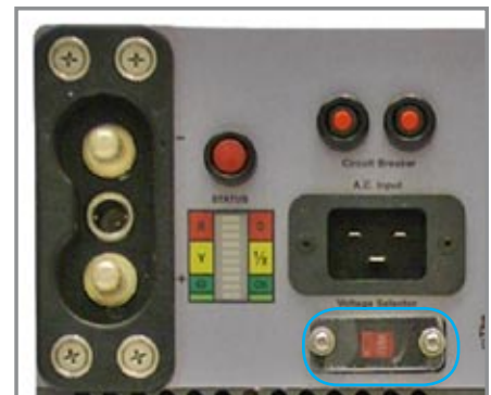
Figure 1.3.4 – TI2500 GPU-24 Input Voltage Selector Switch
