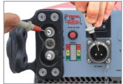
3. Move the positive probe to the dc negative post. Multimeter should read greater than 10\text{ M}\Omega .
