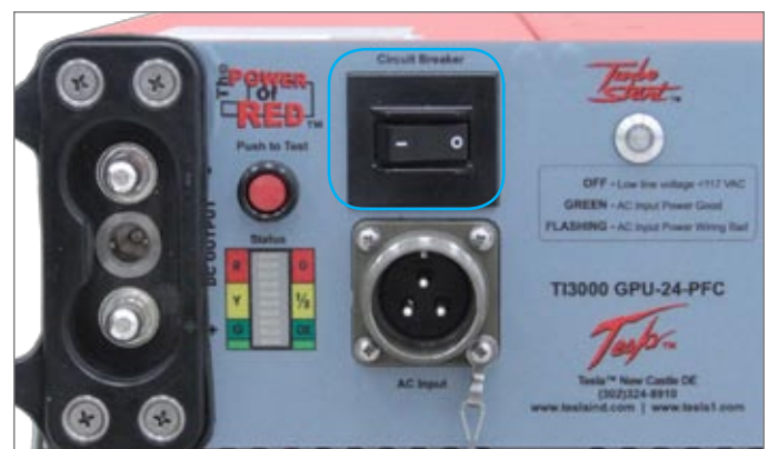
Figure 4.2.1 Circuit Breaker Selector Switch (outlined in blue)
