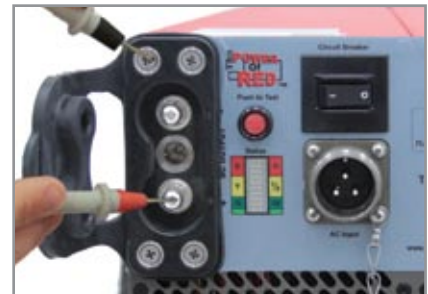
3. Place the negative probe to the fastener screw on the dc receptacle. Move the positive probe to the DC positive post. Multimeter should read 0 Volts.
