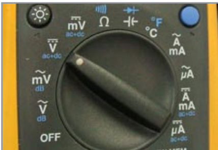
1. Set multimeter to Volts.
