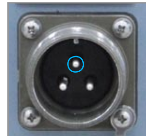
The ground post of the ac input is the middle-top prong (outlined in blue)
