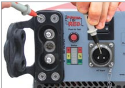
4. Move the positive probe to the fastener screw on the dc receptacle. Multimeter should read less than 1\Omega .
