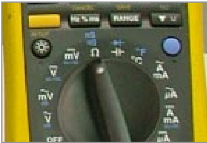
1. Set multimeter to Ohms ( \Omega ).
