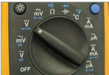
Figure 3.7.5: Set multimeter to Volts.
