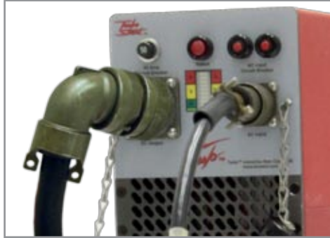
Figure 3.10.1 Attaching DC Power Cable to Unit
