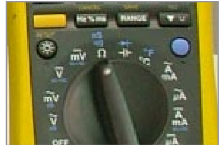
Figure 3.7.2: Set multimeter to Ohms.
