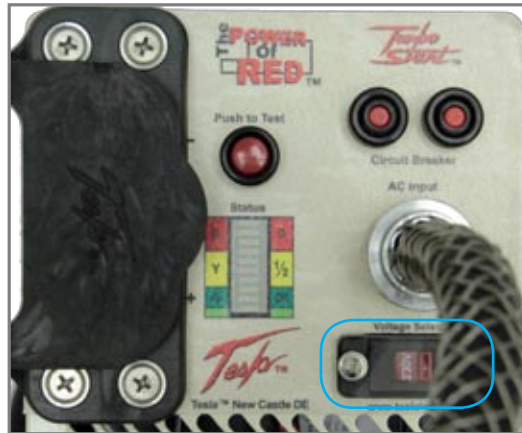
Figure 2.10.1 Input Voltage Selector Switch (outlined in blue)
