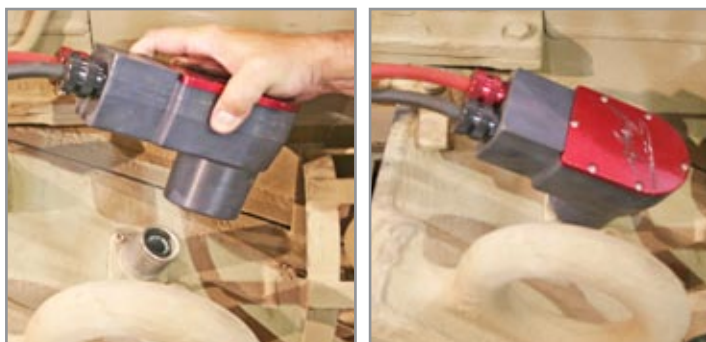
Figure 3.11.2 Attaching NATO DC Power Cable to vehicle
