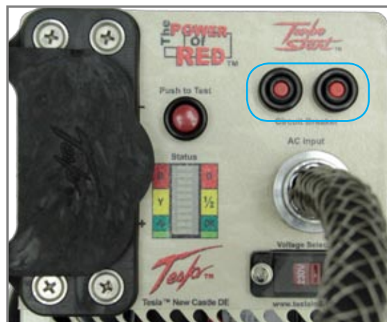
Figure 2.8.1 - AC Input Circuit Breaker (outlined in blue)
