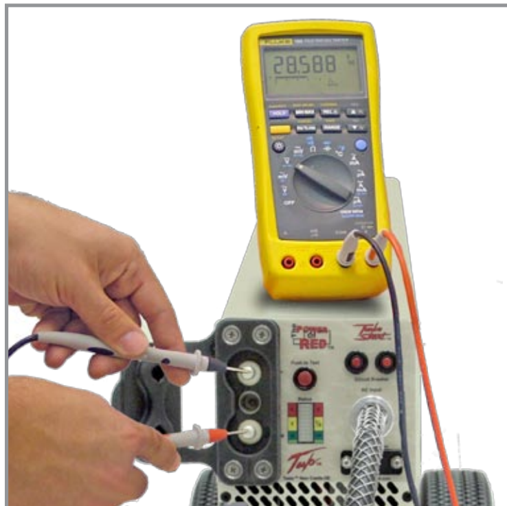
Figure 3.8.2 – Testing DC Receptacle
