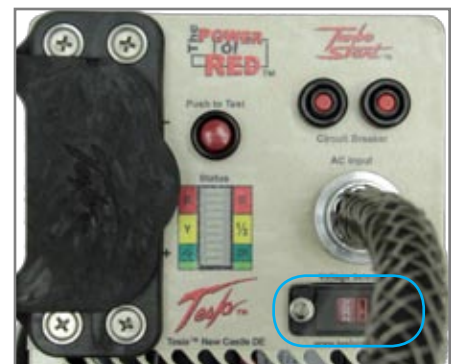
Figure 1.3.4 – TI3000 GPU-24 Input Voltage Selector Switch
