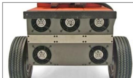
Figure 4.21.2 - Air Exhaust Fans
