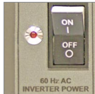
Figure 4.3.2 - 60 Hz Inverter Power Switch
