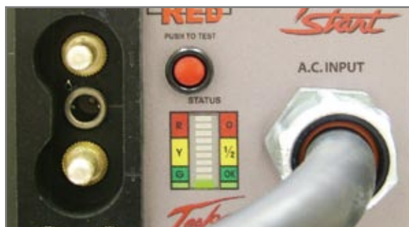
Figure 6.2.1 “Push to Test” and Status Meter
