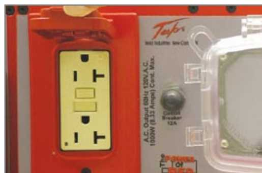
Figure 4.18.2 - 60Hz 120 Vac Output and Circuit Breaker
