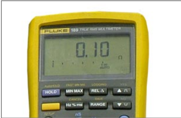
Figure 8.2.6 – Multimeter Reading Continuity (good connection)
