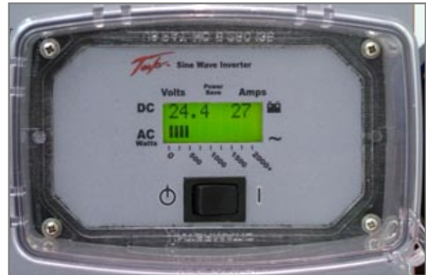
Figure 11.1.5 Inverter Display Panel and On/Off Switch turned on and active.
