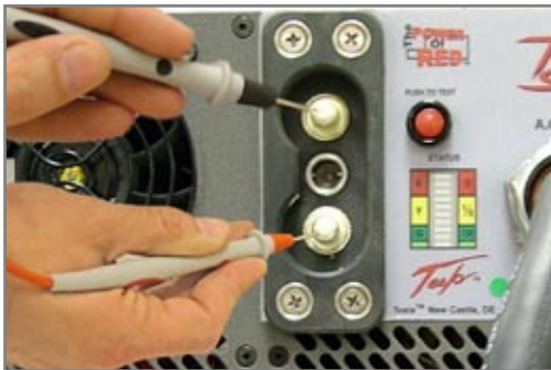
Figure 8.2.16 – Measuring voltage on DC Output Receptacle
