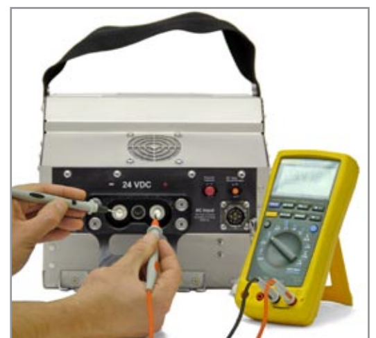
Figure 3.9.3 – Testing DC Receptacle
