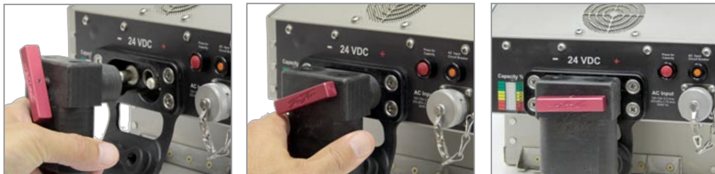
Figure 3.10.1 Attaching dc power cable to TI47407 MPU-24
