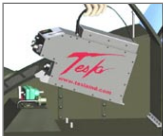
Figure 2.11.1 – Maneuver TI47407 into battery compartment
