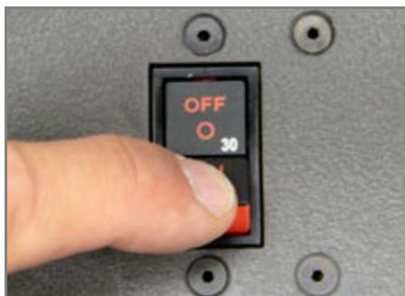
Figure 3.16.6 Switching Circuit Breaker ON
