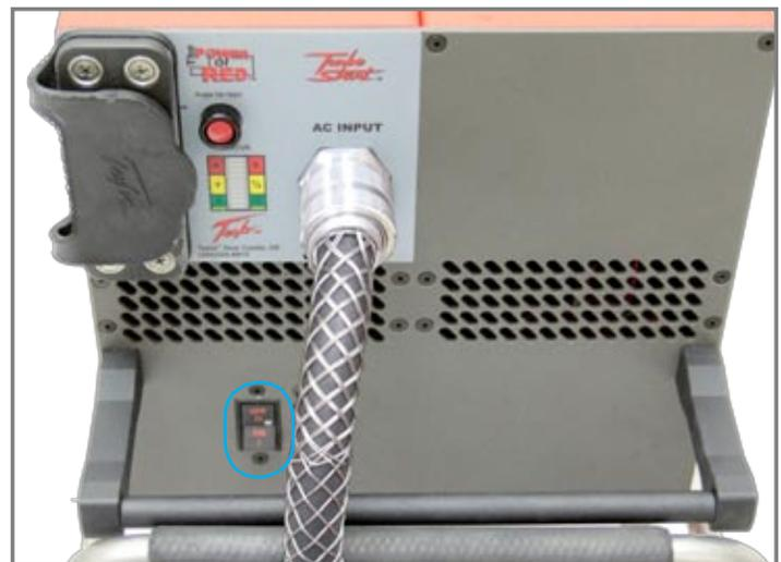
Figure 3.15.1 Circuit Breaker Selector Switch
