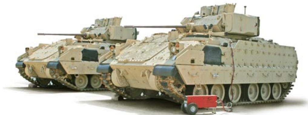
Figure 3.11.3 Starting vehicle with TI4100 GPU-24
