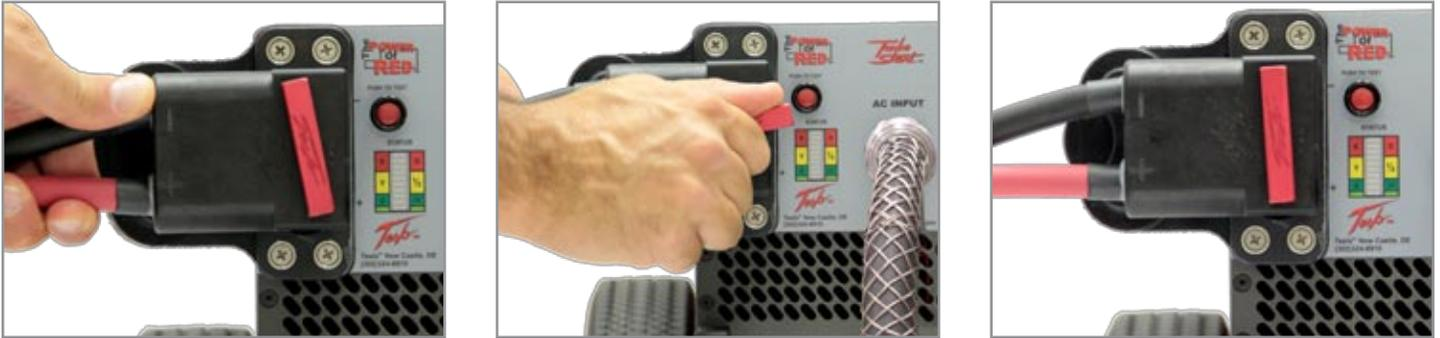
Figure 3.11.1 Attaching DC Power Cable to TI4100 GPU-24
