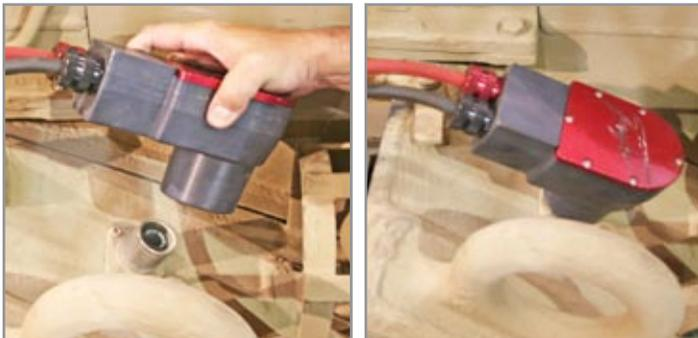
Figure 3.11.2 Attaching NATO DC Power Cable to vehicle
