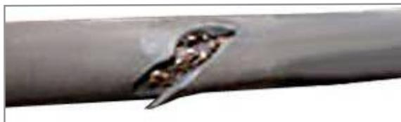
Figure 5.1.1 – Damaged cable
