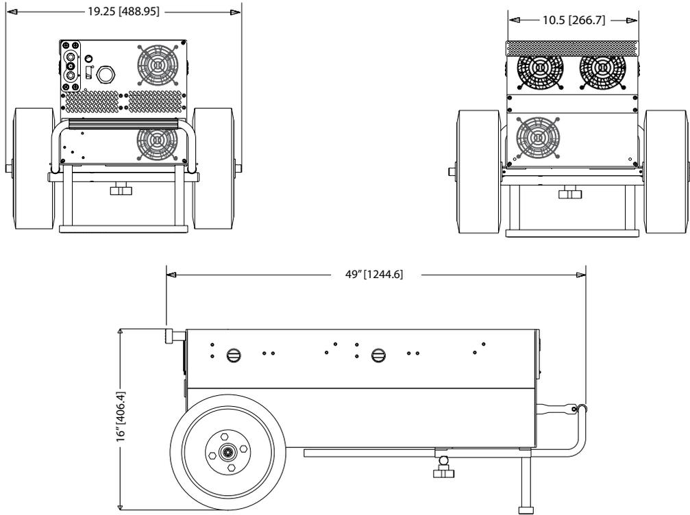
Figure 3.2.1 – TI4200 GPU-24 physical dimensions
