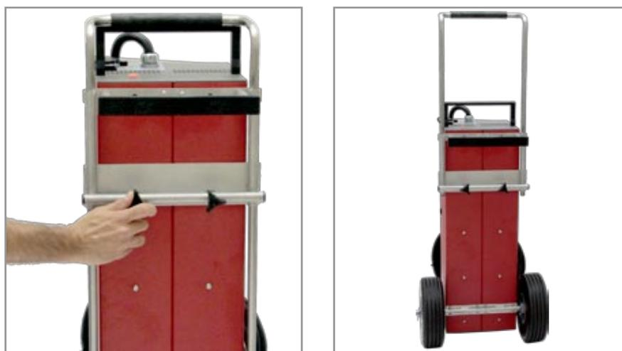
Figure 3.10.1 Releasing Telescopic Handle
