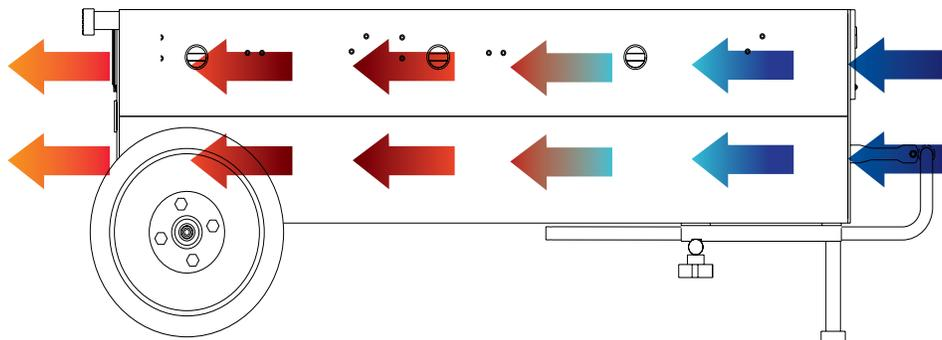
Figure 2.6.1 – Air intake, exhaust ports and internal air circulation
