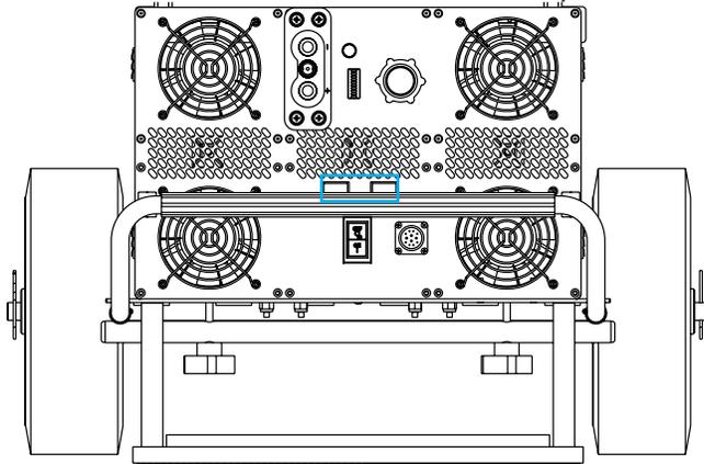
Figure 2.11.1 - Location of the DC Output On and Off Buttons (outlined in blue)
