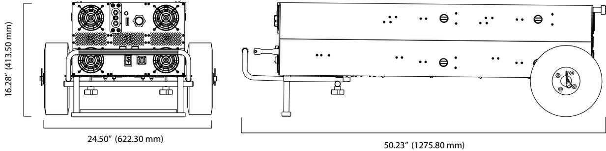
Figure 2.5.1 – TI4400 GPU-24 physical dimensions
