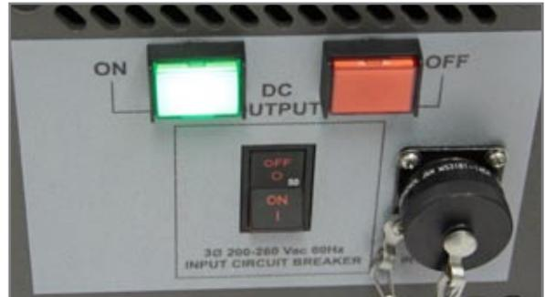
Figure 2.11.2 - DC Output “On” and “Off” Buttons
