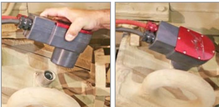
Figure 3.13.2 Attaching NATO DC Power Cable to vehicle
