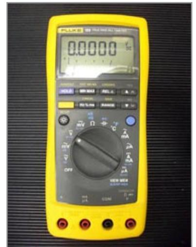
Figure 3.9.1 – Digital Multimeter
