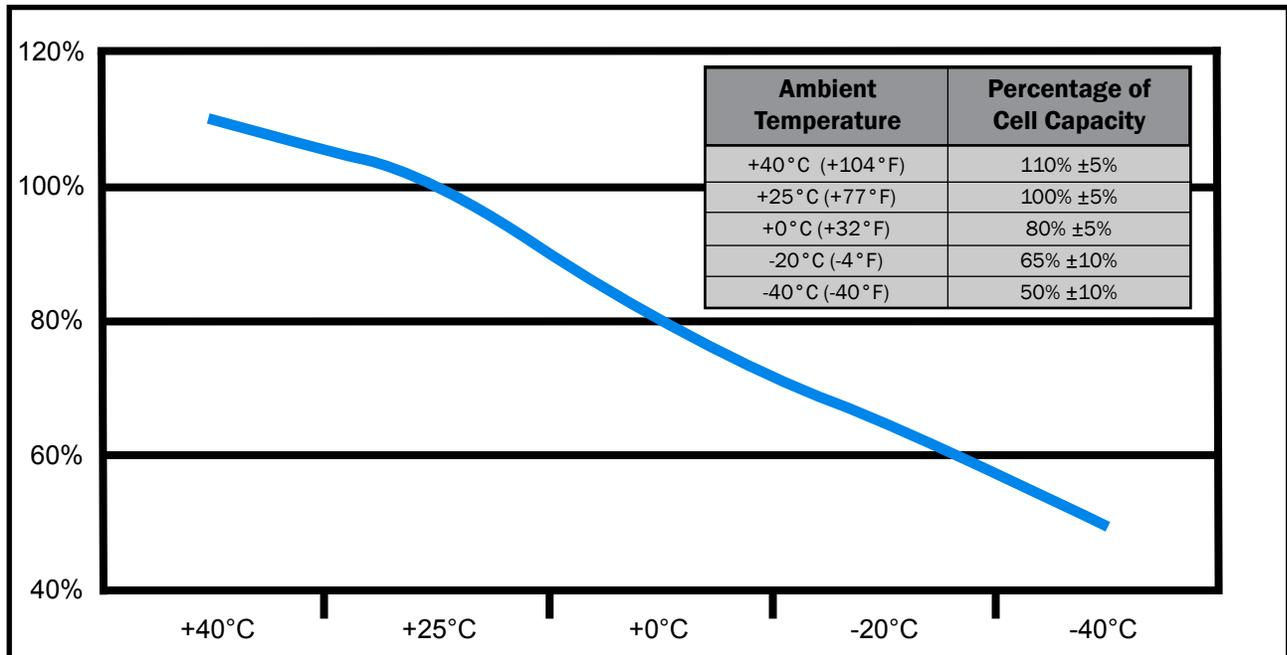
Figure 3.6.1 – Output power capability versus ambient temperature
