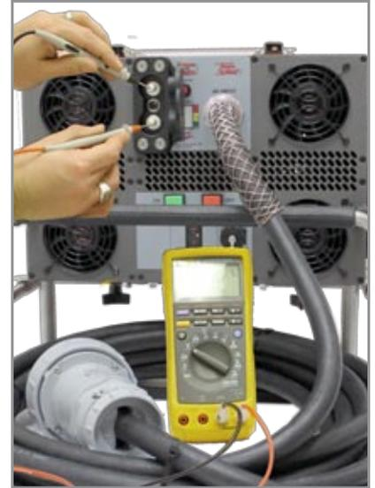
Figure 3.9.2 – Testing DC Receptacle
