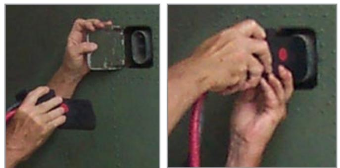
Figure 3.13.3 Attaching an Aviation DC Power Cable to aircraft
