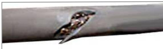
Figure 5.1.1 – Damaged cable
