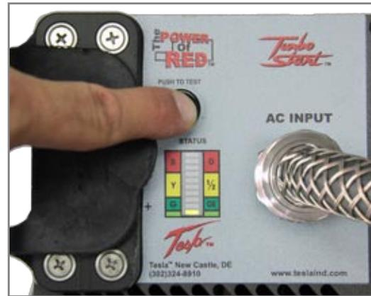
Figure 2.8.1 - Pushing to Test
