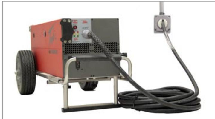
Figure 3.16.4 Plugging Into AC Single Phase Power
