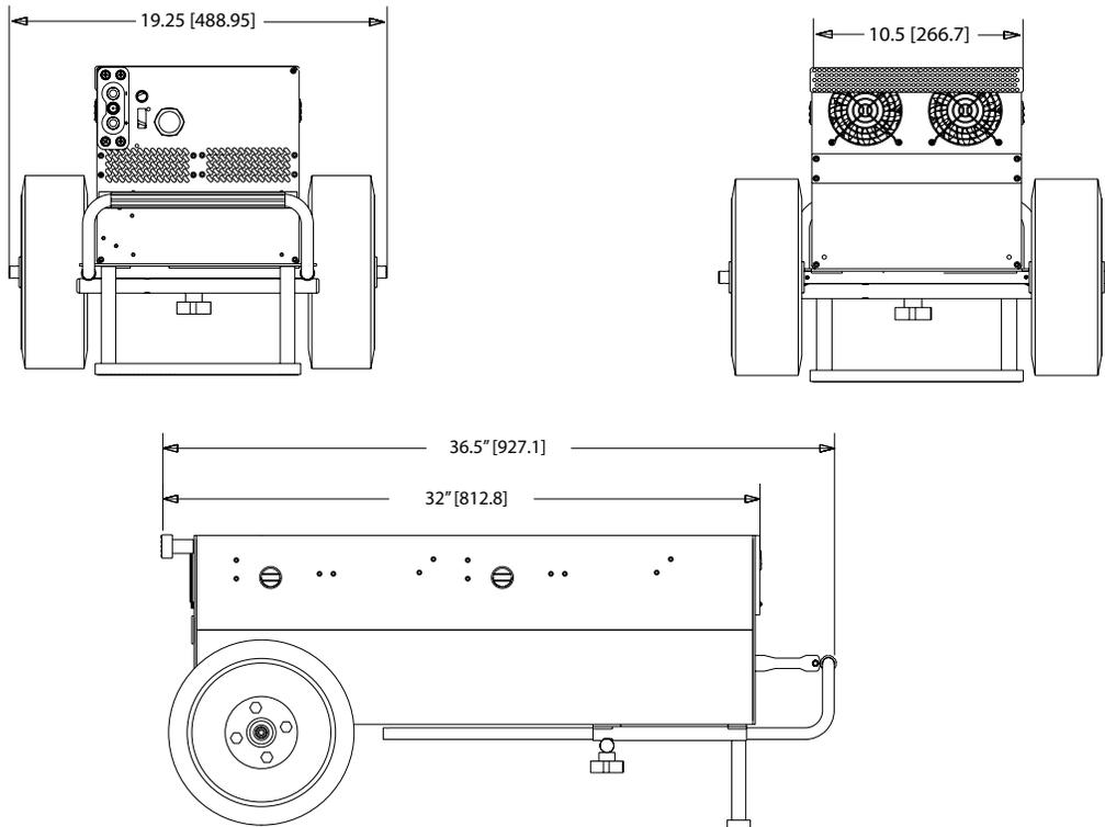
Figure 3.2.1 – TI5100 GPU-24 physical dimensions
