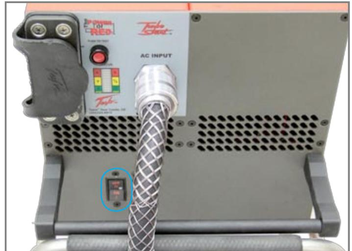
Figure 3.15.1 Circuit Breaker Selector Switch
