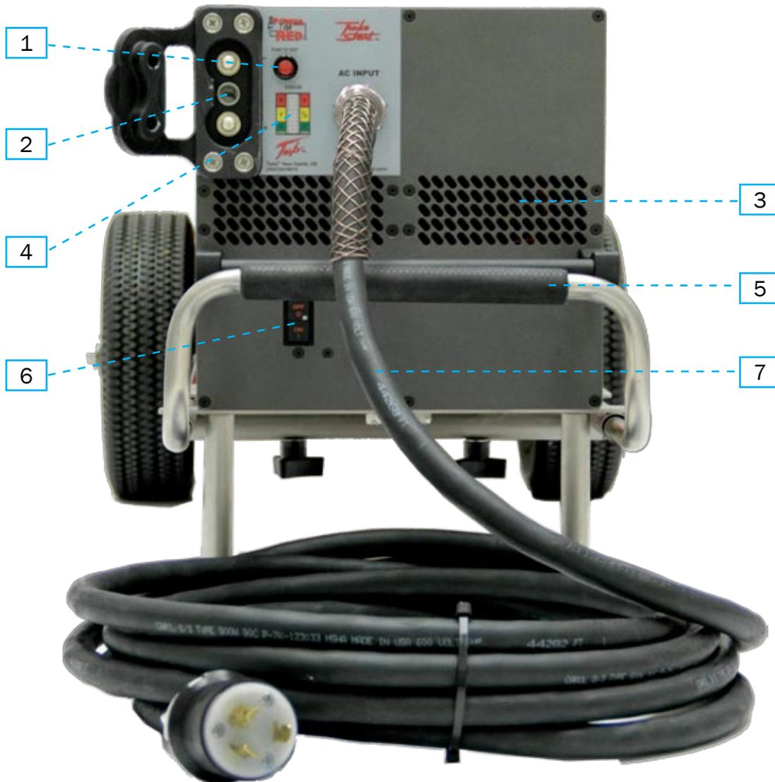
1. **“Push to Test” Button** – Displays current battery charge state when pressed.
