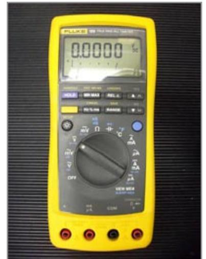
Figure 3.9.1 – Digital Multimeter
