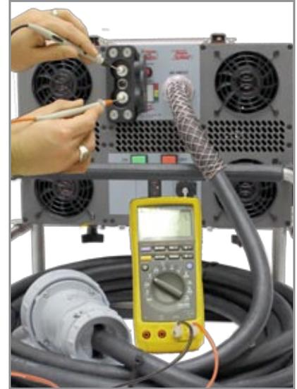
Figure 3.9.2 – Testing DC Receptacle
