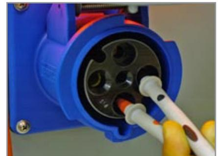
**3.** Move the negative probe to the right side phase 2 probe and the positive probe to lower phase 3 probe.
