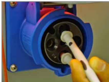
**2.** Move the positive probe to the lower phase 3 positive post.
