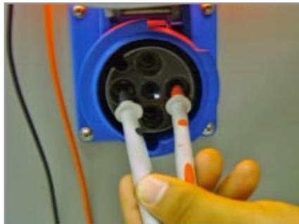
**2.** Move the positive probe to the right side phase 2 positive insert.
